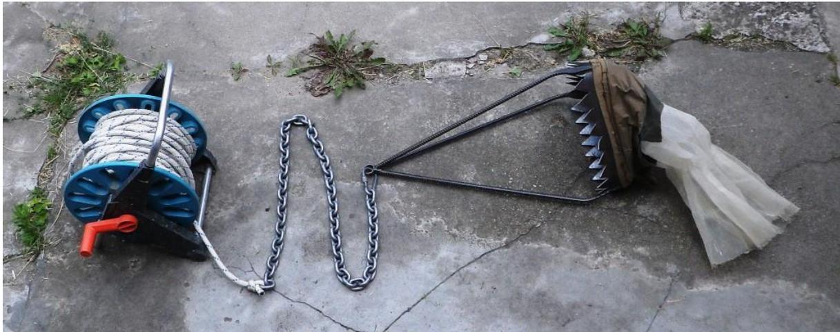
**Figure 3: Bottom dredge with chain and rope for macroinvertebrate sampling**
