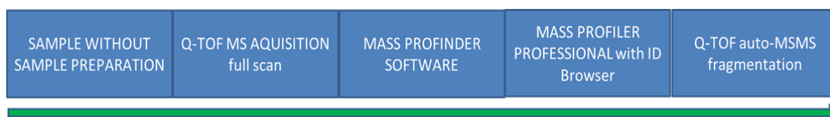
Figure 1 Non-target workflow used for analyses by UHPLC-Q-TOF-MS
