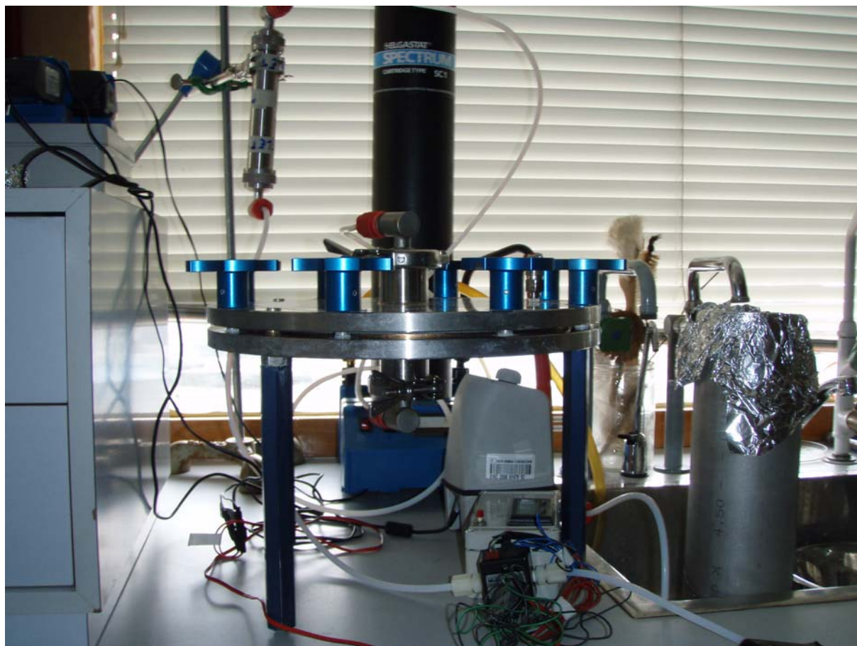
Figure 2.1.2-1 Large volume sampling device – Filter/XAD system
