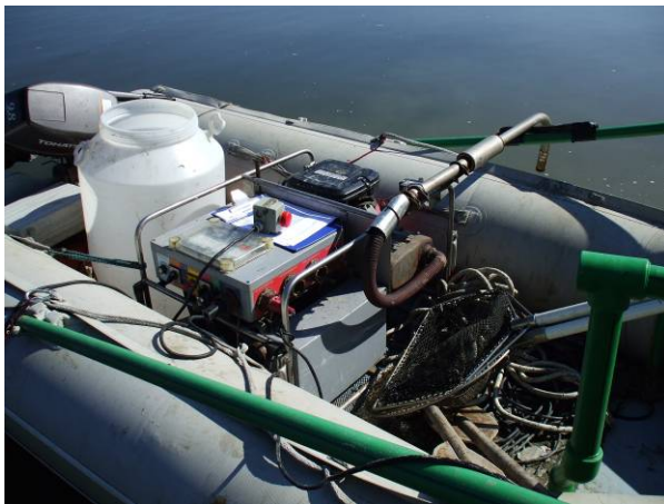
Exhaustion tube, electric generator and on board fish tank (left) and land based fish tanks with freshwater pump (right)
