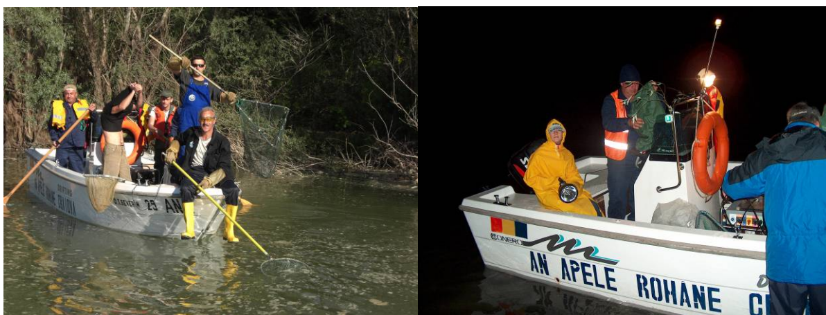
Electro fishing with handheld anode (left) and spotlight and torches used for night sampling (right)
