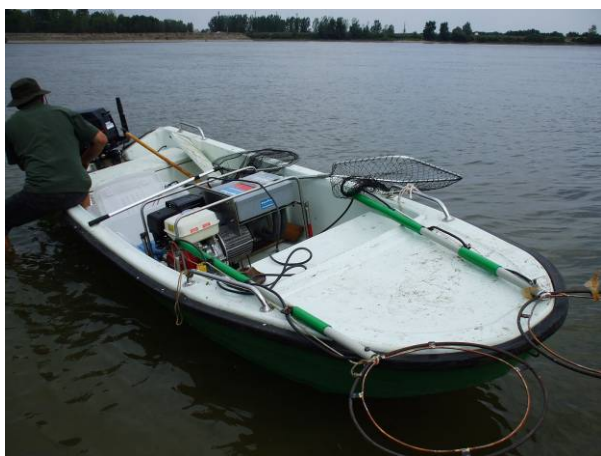
Two handheld anodes (only one was finally used) with only partially isolated sticks
