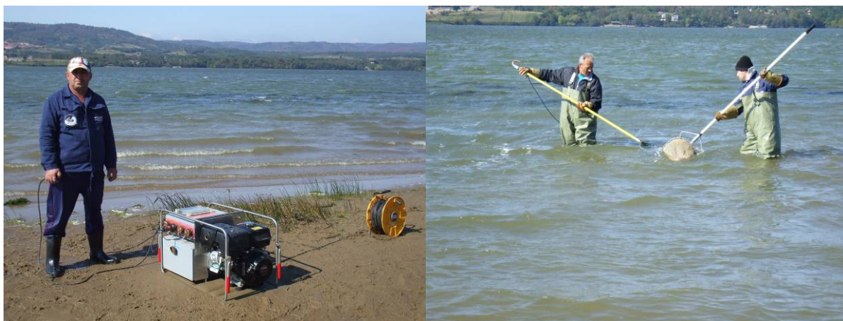
Electric generator and cable roll (left) used for electro fishing by wading with handheld anode (right)
