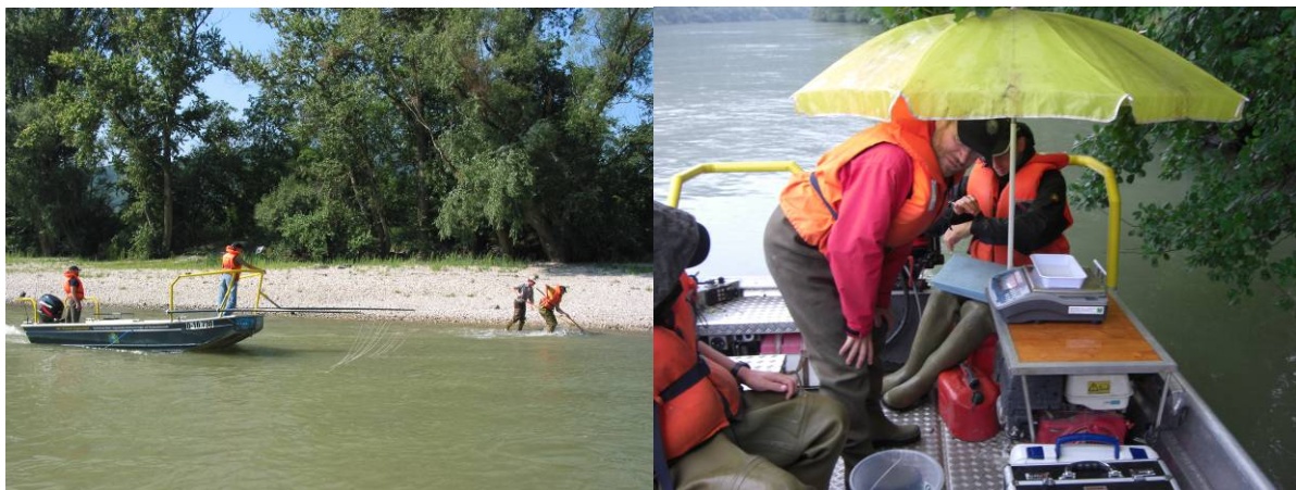
Electro fishing by wading with handheld anode on long cable (left) and protective working table with scale on boat (right)
