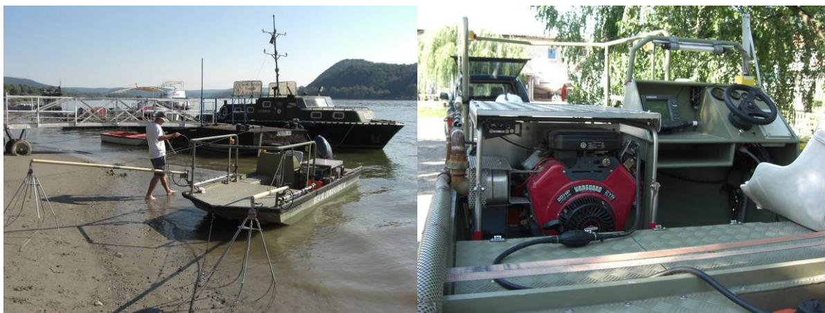
“Spider” boom anode (left) and protective/working table with steering console (right)
