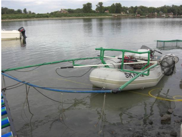
Boom anode (left) and plastic tube railing (right)
