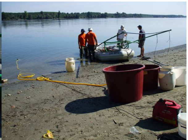
Exhaustion tube, electric generator and on board fish tank (left) and land based fish tanks with freshwater pump (right)
