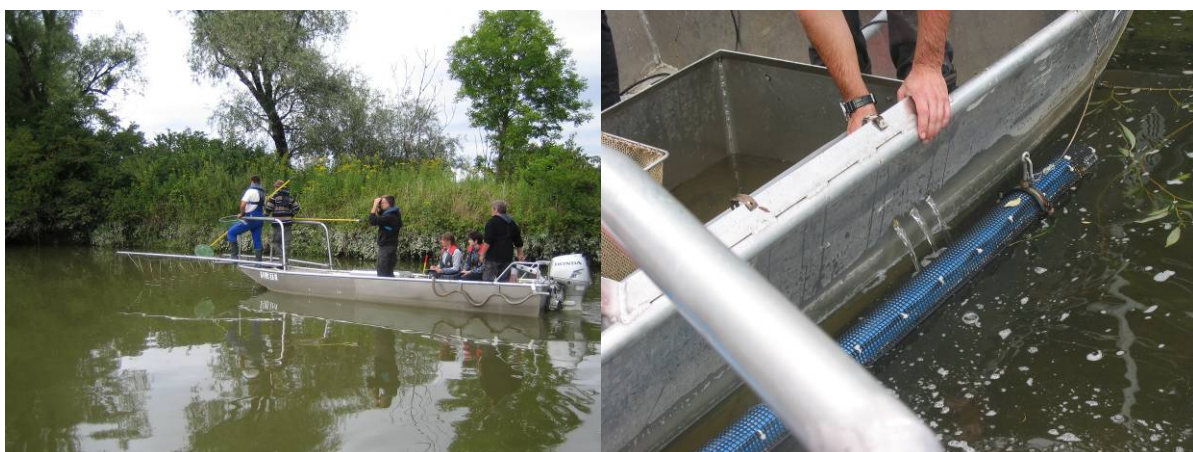
Boom anode fishing (left) and outlet of fish tank with permanent freshwater supply and floating cathode (right)
