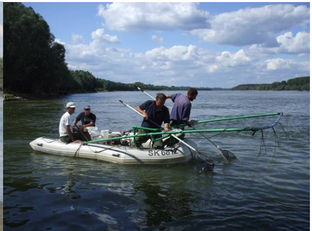
Electro fishing by wading with handheld anode (left) and by boat with boom anode (right)
