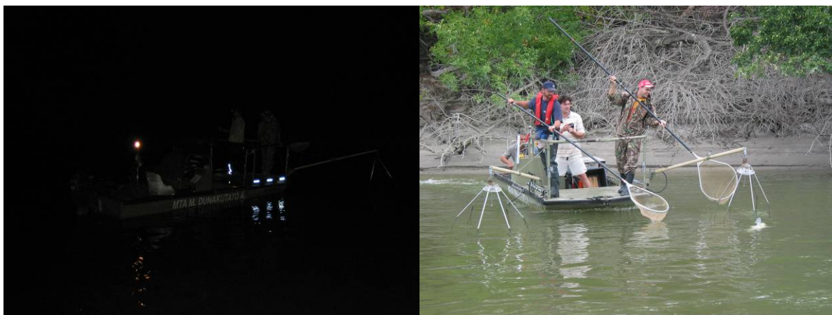
Night sampling using LED lamps (left) and electro fishing with boom anode (right)
