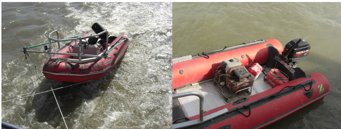
Zodiac tied at rear end of Vienna 115 for transport (left), electric generator, outboard engine with tank and battery (right)
